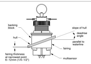
Figure 2. Deadrise angle & fairing thickness (B66V shown)
