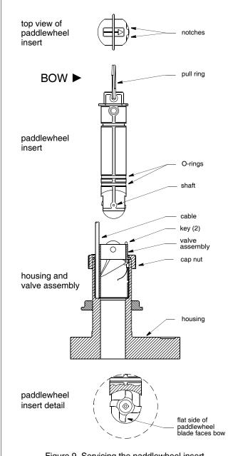
Figure 9. Servicing the paddlewheel insert and the valve assembly (B744V shown)
